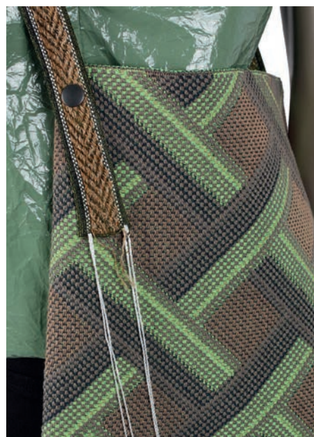
Single jersey tote bag with multiple weft insertions and STOLL-ikat plating® graphic in geometrical lattice design.
